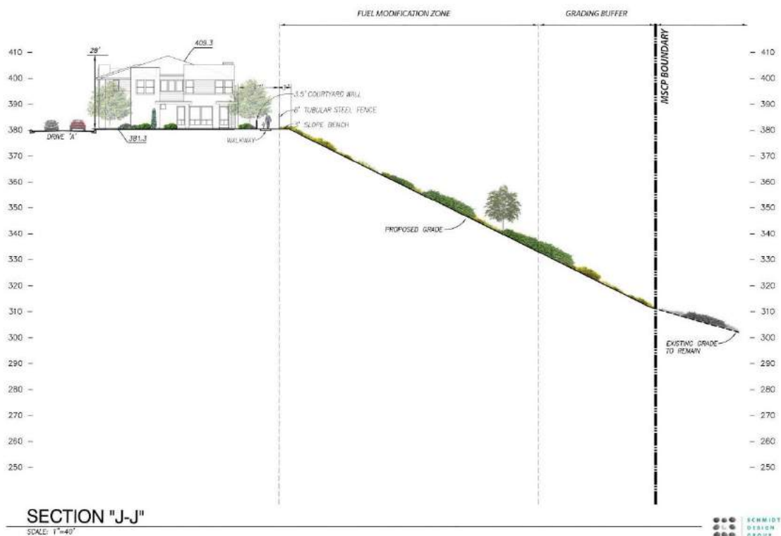
Exhibit 26: Perimeter Edge Condition @ R-1 (Cross Section J-J)
